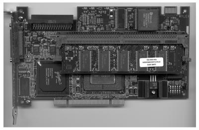
Figure 1-1. AcceleRAID 170 Controller
